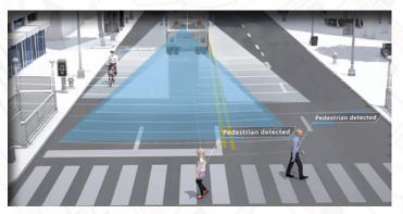
In addition to all the benefits of the original Mobileye® Collision Avoidance System, this unique, smart vision multi-sensor system provides drivers with alerts when pedestrians and cyclists are in the danger zones on the side of the waste truck as well as the front. Often times, pedestrians will dart out between cars to cross the street and into a driver's blind zone. Shield+can minimize such safety concerns. The addition
