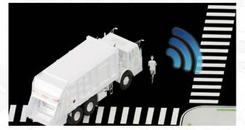
The optional "intelligent", external alert system will send an audible alert to VRUs around the bus to ensure they are aware that the bus is within the vicinity and maneuvering around them. The alert will <u>ONLY</u> sound when Shield+ detects an imminent collision between the vehicle and a VRU. This "intelligent" or smart technology alert reduces noise pollution and helps prevent VRUs from "tuning out" excessive alerts that sound at every turn.
